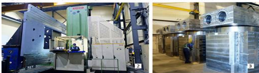
Manufacturing of the 10,000 Ton Presses: Image 1 - HPU at Macrodyne's Racco Facility. Each HPU will have 4 x 400HP pump motor groups with high-pressure closed loop piston pumps that will deliver up to 600 Liters per minute of hydraulic oil at 7250 Psi. Image 2 - Machining the frame plates(1 of 6) at Macrodyne's Concord facility that will form the frame of the press. Each frame with the bolster will weigh 830,000 Lbs, and will be 195" wide x 395" high x 105" deep. Image 3 - Cylinders during the manufacturing process. Each cylinder weighs 165,000 Lbs, and has a bore diameter of 59.25".
