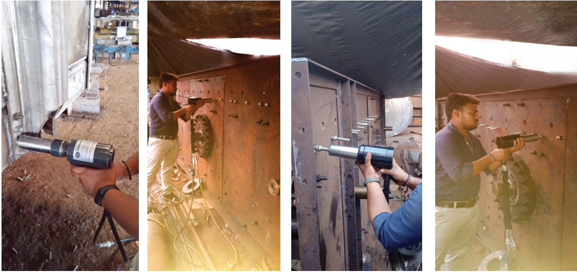
STATIC HYDRAULIC MAKE LOCK BOLT INSTALLATION TOOL AT WAGON And VIBRATING SCREEN MANUFACTURING
